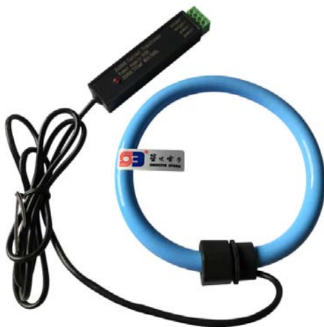
0.333Vac output with integrator
