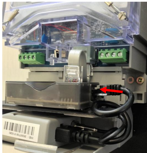
4. Connect the modem to the Integrator.
